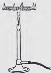
FIG. 9.—Action of Wire Gauze on Flame.
